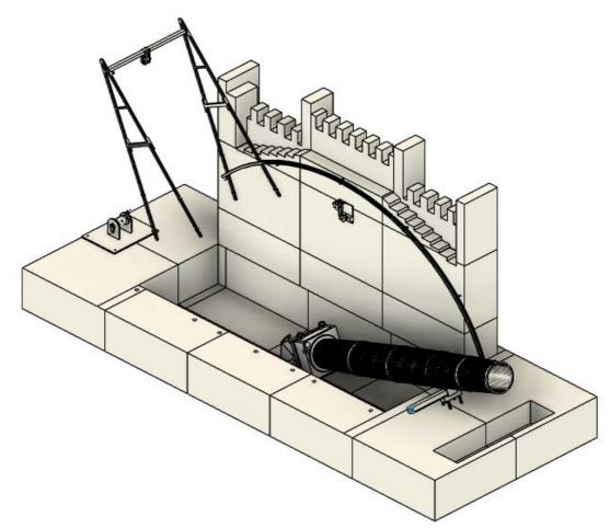
Towards the front of the telescope tube is a rectangular steel tube at 90 deg to the tube axis. Through this runs a beam that is loosely attached to the arced rail on the right wall. When the front of the tube is raised then the beam follows the arc. Gearing within the steel box and rods up to the observer allow the observer to track a target in azimuth.
